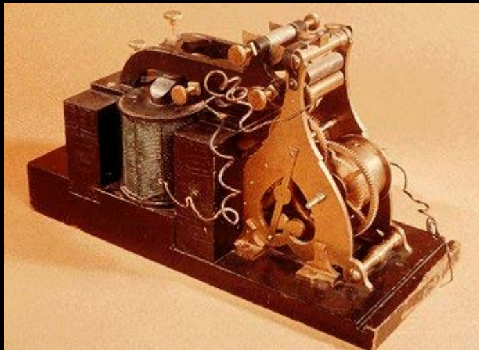
Samuel Morse Telegraph Receiver – Used to receive the message, "What hath God wrought" during the demonstration to Congress in 1844.
