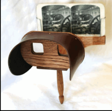
Sir Charles Wheatstone, stereoscope, 1840
